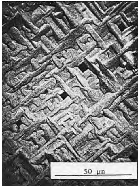
Figure 4.125 Light micrograph of the as-grown surface of a film of GaP grown on (100) oriented Si. (After Morizane 1977. Reprinted from Journal of Crystal Growth , 38 , Antiphase domain-structures in GaP and GaAs epitaxial layers grown on Si and Ge, pages 249–54. Copyright 1977, with permission from Elsevier.)
