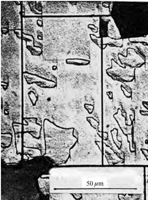
Figure 4.117 Light micrograph of an etched surface of a film of GaP epitaxially grown on a (100) surface of NaCl and floated off in water. The APBs appear as irregular closed curves. The straight vertical and horizontal black lines are cracks. The cracks run straight across the APBs because the orientations of both domains are the same, i.e. the Friedel index of the APBs is \Sigma = -1 . (After Morizane 1977. Reprinted from Journal of Crystal Growth , 38 , Antiphase domain-structures in GaP and GaAs epitaxial layers grown on Si and Ge, pages 249–54. Copyright 1977, with permission from Elsevier.)
