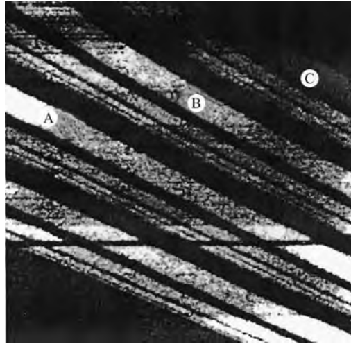
Figure 3.15 Panchromatic STL image of a cross-section through four sets of different GaAs/ \text{Al}_{0.38}\text{Ga}_{0.62}\text{As} QWs with different doping density at 300 K. The area of the image is 1.73 \times 1.73 \mu\text{m}^2 . (After Alvarado et al. 1991. Reprinted with permission from Journal of Vacuum Science and Technology , B9 , pp. 409–13. Copyright 1991, American Institute of Physics.)
